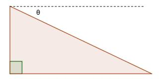
The angle of depression is the angle formed by the line of sight and the horizontal plane for an object below the horizontal.
