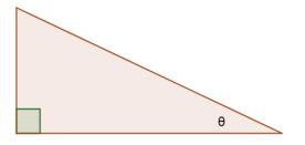
The angle of elevation is the angle formed by the line of sight and the horizontal plane for an object above the horizontal.
